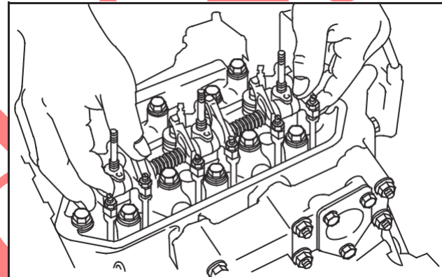
Fig. 35 – Install Rocker Arm Assembly
